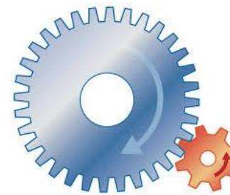
**Gears** are toothed wheels which lock together and turn each other to form simple machines.
